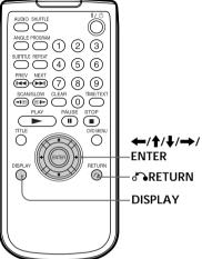
Press DISPLAY and select "SETUP" using ↑/↓.
